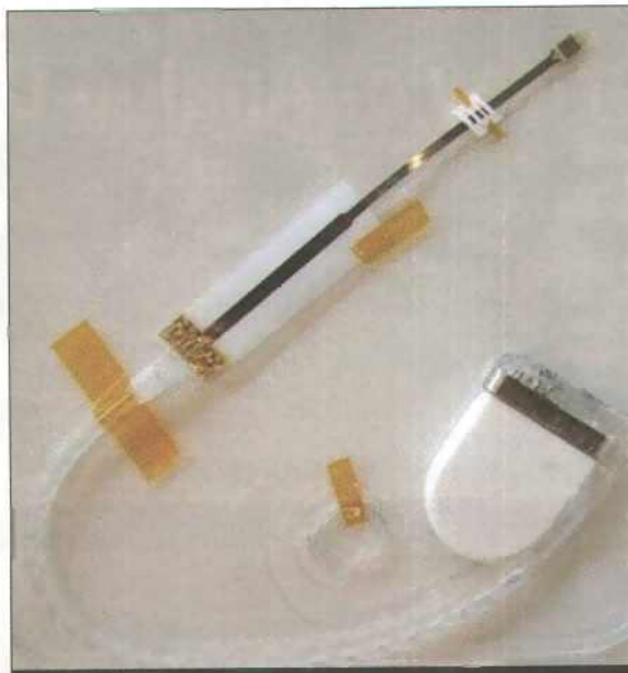
University of Ulm prototype artificial retina comprises an implantable chip and a controller worn behind the ear.
